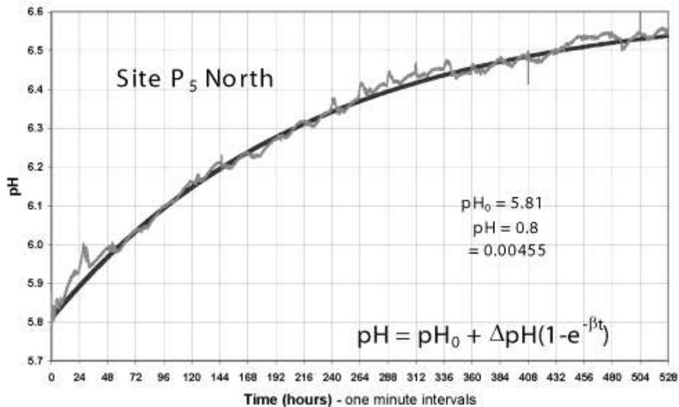
Figure 5b. pH vs. time at control site P<sub>5</sub> North room.
